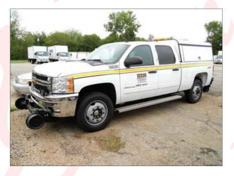
The Track Inspector makes riding down the rails in a Ford or Chevrolet pickup truck simple.
